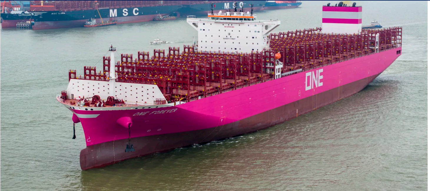
SUZHOU, CHINA - MARCH 18: 'ONE FOREVER' container ship, with a length of 366 meters and width of 51 meters, is assisted by tugboats as it prepares to leave a dockyard of Jiangsu Yangzi-Mitsui Shipbuilding Co., Ltd. on March 18, 2024 in Suzhou, Jiangsu Province of China.
